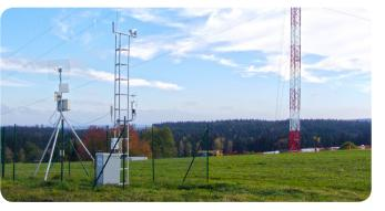
This Ecosystem Station uses a standard methodology (eddy covariance) to monitor matter and energy fluxes between the local agroecosystem and the atmosphere. Micrometeorological and biomass parameters and nutrient contents are measured, too.
